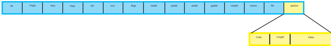
Figure 16-1. DHCP Packet Format
